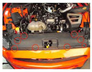
**Step 3:** Remove the 8 bolts securing the bumper cover to the radiator support.
