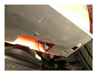
**Step 3:** Prep the tape mounting surface with the supplied alcohol swabs and adhesion promoter.
