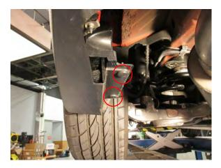
**Step 7:**Secure with factory plastic push clips. \*\*Note: push clips will be tight and will require more pressure to seat the clip.
