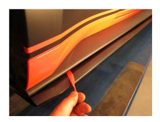
**Step 5:**Locate and remove the two plastic push clips that fasten the rear bumper.
