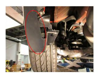
**Step 8:**Peel the plastic backing film, and firmly press the rear splitter to the bumper.
