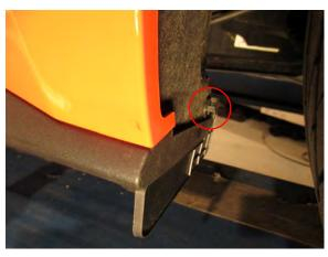
**Step 2:**Remove the 8 clips securing the plastic radiator cover to the support and remove it from the vehicle.
