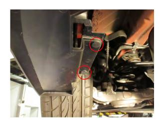
**Step 6:** Clean the area the tape will mount to using the supplied alcohol swab and adhesion promoter.
