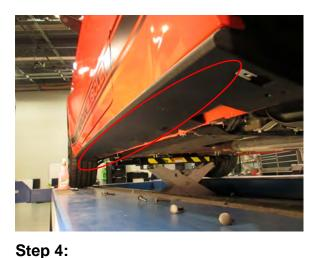
Peel back the red plastic film to expose the double sided tape. \*\*Note: only peel off enough to get it started. Install the Rocker splitter using the factory retaining clips. Once the splitters are where you want them, peel the red film off and apply firm even pressure.
