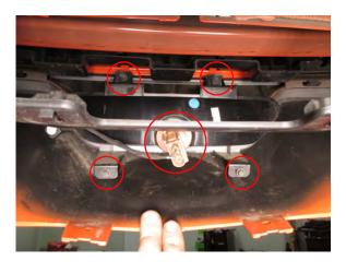
**Step 5:** Apply firm pressure to remove the factory trim tabs from the bumper.
