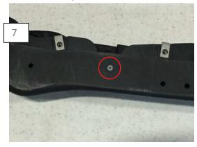
Remove the chin spoiler brace from the chin spoiler by drilling out the rivet. \*\*Note: This will NOT be riveted to the Foose chin spoiler.
