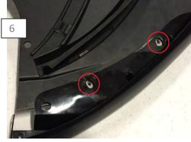
Non-Track Pack Cars, Reinstall the splash shield using the factory holes. Secure the outer splash shield to the Foose lip using these holes on both sides.
