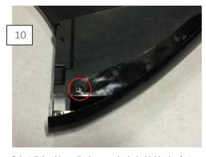
Reinstall the chin spoiler brace and splash shield using factory hardware. The outer edge of the splash shield will only be secured to the Foose chin spoiler using the hole circled above.
