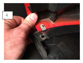
Install the screw clip on the bumper cover as seen above.
