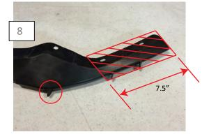
Measure 7.5" from the end of the chin spoiler brace and cut a straight line. Remove the plastic nipple from the brace circled above. \*\*Note: Performance Pack cars only.
