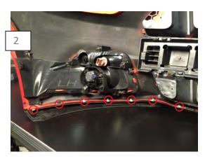
Remove the fasteners holding the chin spoiler to the bumper. Base and Performance pack cars are secured using similar hardware.
