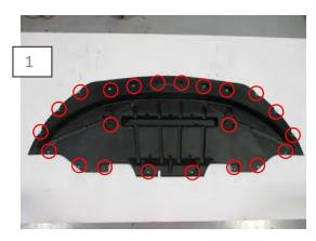
Support the front of the car so you can access the bumper splash shield. \*\*Note there are two versions of the splash shield (Track Pack and Non Track Pack). Both are attached to similar locations
