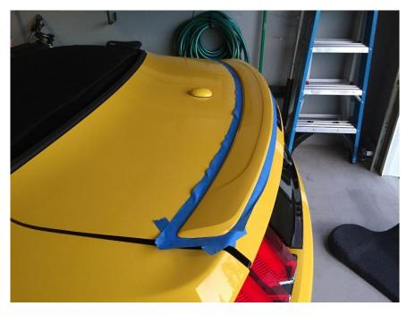
Step 4: Use painter's tape to mask off the edges of the factory spoiler to protect your trunk lid paint.
