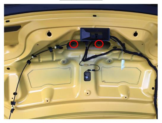
Step 3: Using a 10mm Deep Socket and ratchet, remove the 4 nuts on each of the 4 mounting studs for the factory spoiler. One can be found under the grommets removed in Step 2. The last 2 can be found behind the high mount brake light near the center of the trunk lid. (pictured above)
