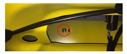
Step 17: Begin mounting the MMD by Foose spoiler, starting with the two inner most screws. Hand tighten to start but DO NOT fully tighten the screws yet.
