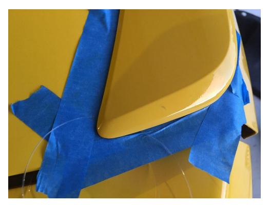
Step 5: Beginning on either end of the factory spoiler, run fishing line under the corner of the spoiler (heavier gauge or "big game" fishing line – as mentioned in the tools section – will be less prone to breakage and make this process much easier!) Slowly move the line back and forth until you can go no further (this means you will have hit the outer mounting studs) This process will help separate the factory double sided tape.
