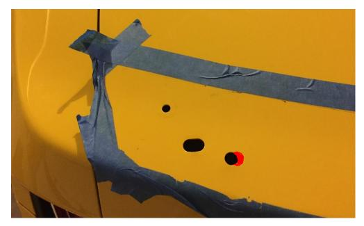
\*\* For cars WITH a factory spoiler, begin by drilling a pilot hole in the center of both MIDDLE templates (closest to the brake light) Continue drilling, finishing with a ¼ inch bit.
