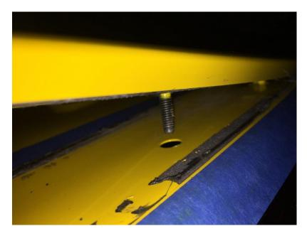
Step 7: Continue sawing back and forth with the fishing line until you reach the inner mounting studs. Gently pull up on the spoiler to expose the studs and feed the line under. Repeat with each stud until you have cut through to the other side. Now carefully remove the factory spoiler.
