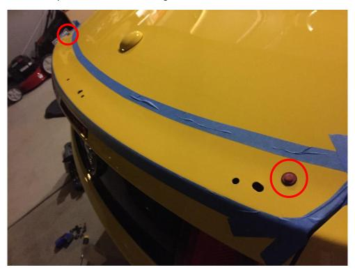
Step 9: Remove the factory mounting plugs (pictured above) with a trim removal tool or needle nose pliers. Be sure to tape around them to protect your paint during removal. Clean any dirt with a microfiber towel. Your factory spoiler removal is now complete!
