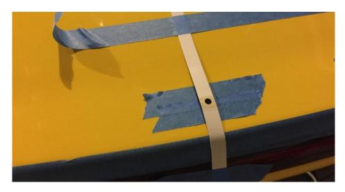
Step 13: \*\*For cars WITHOUT a factory spoiler, begin by drilling a pilot hole in the center of each template. Continue drilling, finishing with a ¼ inch bit. NOTE the MMD instructions will say finish with a 7/32 bit. I found this was a bit tight fitting around the new hardware and a ¼ bit worked best. For additional protection, place a small block of wood beneath the outer drill spots to make sure the bit does not contact the top of the tail light housing.
