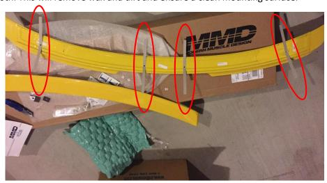
Step 11: Using the supplied mounting templates, locate the 4 mounting points on the bottom of your MMD by Foose spoiler. Center the mounting templates over each and apply. There is an adhesive section of each template near the drill hole. This is the MOST IMPORTANT step for drilling accuracy.
