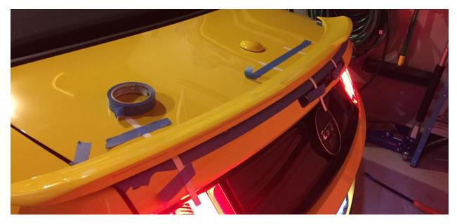
Step 12: Center and test fit the MMD by Foose spoiler. BEFORE securing each template, you will want to add painters tape beneath each template to the trunk lid to protect your paint from cracks while drilling. (see next picture for example) Now secure the templates to the car as shown above with painters tape. Carefully pull the MMD by Foose spoiler away to reveal your drilling templates.
