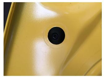
Step 2: remove the factory rubber grommets from the driver and passenger sides of the trunk. This can easily be done by hand. On models equipped with a factory spoiler, this will expose a mounting stud on each side. (see picture on right)
