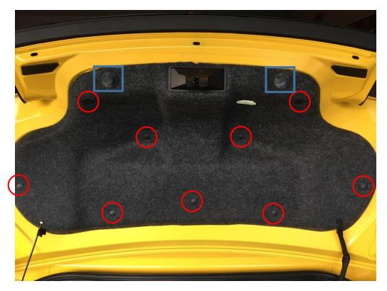
Step 1: Remove the trunk inner liner. There are 9 panel screws (red circle), 2 trunk stops (blue square) that will need to be removed. Use a trim removal tool or needle nose pliers to remove the trim screws. The trunk stops can be removed by hand by turning counter-clockwise. Once complete, the trunk liner can be removed by slowly working it around the trunk latch. The emergency trunk release can simply be popped through the trunk liner by hand to be removed.
