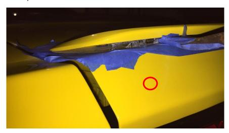
Step 6: Gently pry up on the edge of the factory spoiler. You will need to feed the fishing line around the factory mounting studs (near circle above) on the outer edge of the spoiler to continue cutting through the double-sided factory tape. I found a trim removal tool wrapped in painters tape to protect from sharp edges to be the best at holding the spoiler up while feeding the line.
