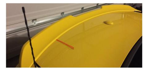
Step 18: Peel back the double-sided tape protector and firmly press the MMD by Foose spoiler to the trunk surface. Finish by installing the last two mounting screws on the outer most mounting holes. Tighten all mounting screws down with a Phillips head driver.
