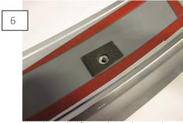
Place the supplied foam pads over the mounting holes on the spoiler. Trim as need. Remove tape backing and install the wing using the provided hardware.
