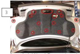
Remove the deck lid panel. There are various push pins, the rubber bumpers located at the top unscrew. I was able to sneak the liner off by manipulating it around the latch trim.
