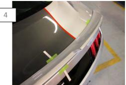
Test fit the spoiler and center it on the deck lid. Then tape the template to the deck lid where they lay. Carefully remove the spoiler from the templates. \*\*Note: this is the most important step so that the holes are drilled in the correct place.
