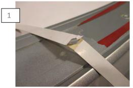
Using the provided drill template. Remove the center adhesive contact. Place the adhesive side on the spoiler, centering it over the bolt hole.
