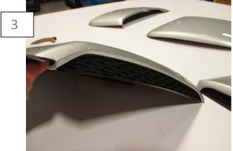
Remove the tape backing from the insert and install the insert to the louver.
