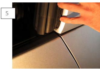
Remove tape backing. Line up the bottom, front, top edges and apply to glass.
