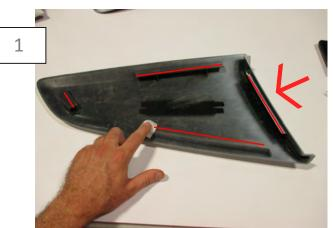
Wipe the tape ledges on the louver and window glass with provided alcohol wipes followed by adhesion promoter. \*\*Note: A clean surface is essential for proper adhesion.
