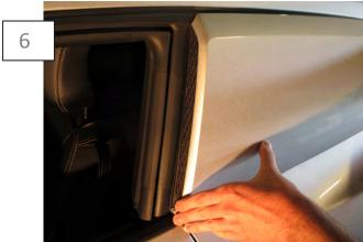
Once placed, apply firm pressure over all tape surfaces.
