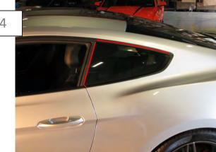
Fit the part before removing tape backing. The leading edge of the insert sits flush against the weather stripping. The top edge of the louver follows the indent on the window molding.
