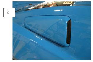
Test fit the scoop and note how the scoop fits to the window. Then remove tape backing, apply the scoop to the window using firm even pressure.
