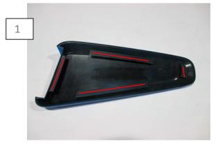
Wipe the tape ledges on the Scoop and window glass with provided alcohol wipes followed by adhesion promoter. \*\*Note: A clean surface is essential for proper adhesion
