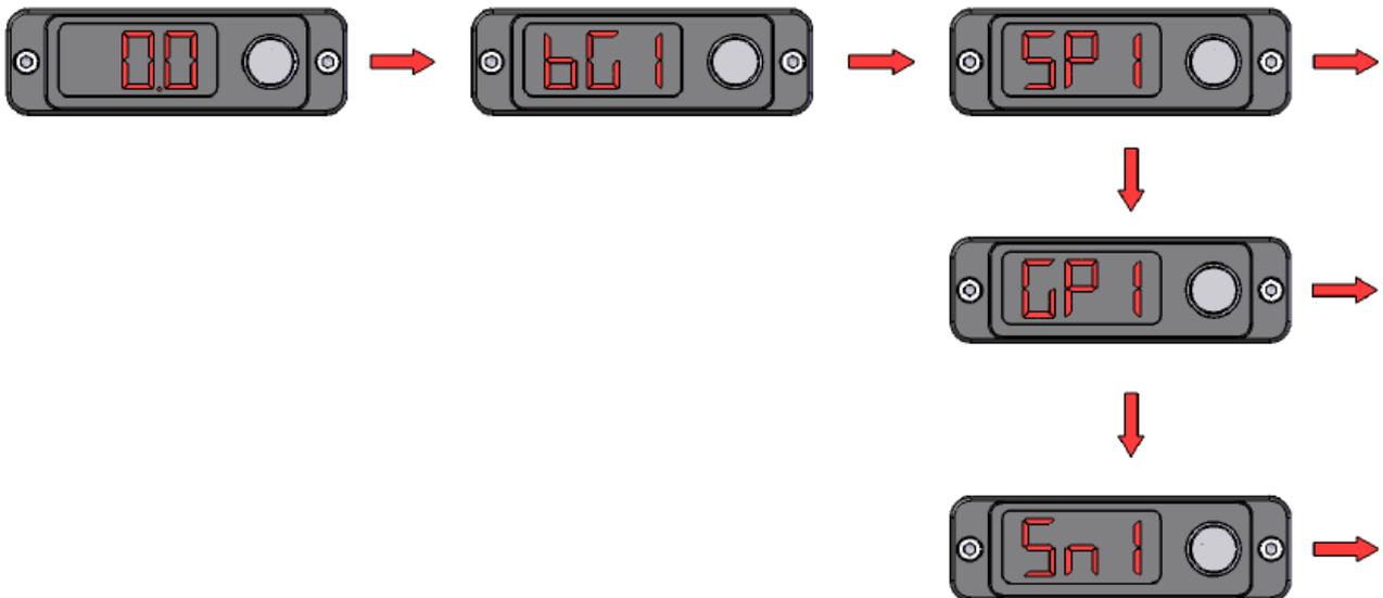
The E-Boost Street has the ability to control two levels of boost (BG1/BG2). The parameters that can be adjusted in each boost group are set point (SP1/SP2), gate pressure (GP1/GP2) and sensitivity (SN1/SN2). Set up the boost groups in the following order:
