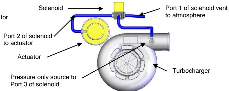
If you are unable to achieve your desired boost pressure, it is normally due to exhaust manifold backpressure forcing the internal waste gate to open. To increase your boost pressure further, fit a higher pressure waste gate actuator to increase your minimum boost pressure.
