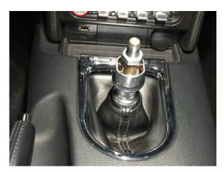
Install the supplied nut. This nut is used to align the shift pattern on the shift knob. Thread the shift knob on until it is tight against the nut. If the shift pattern does not line-up simply adjust the nut up or down until it does. \*\*Note: Ensure the reverse lockout is still functional. If not, loosen the lock nut and knob until it does.
