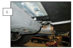
Mount the lower tabs by first removing the 11mm bolt, installing the tab and then press the tab against the diffuser.
