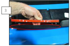
Prep the Diffuser with the alcohol wipe and adhesion promoter anywhere that the diffuser tape makes contact to bumper.
