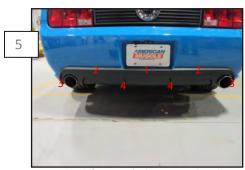
Center the diffuser on the bumper and apply firm even pressure on tape surfaces. Following the above sequence.
