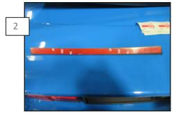
\*\*Note the Orientation of the mounting tab, they are side specific. This is the left side.
