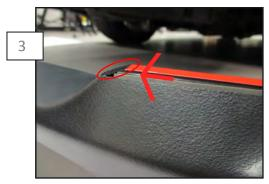
Prep the Diffuser with the alcohol wipe and adhesion promoter anywhere that the diffuser tape makes contact to bumper. \*\*Note how the tape ledge is flush with the diffuser cut.
