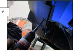
Once the diffuser is mounted, drill a 7/16th hole through the bumper cover and install supplied push clip.
