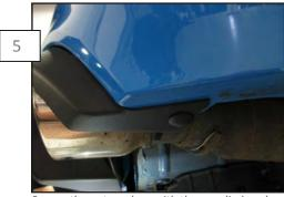
Secure the outer edges with the supplied push clips.
