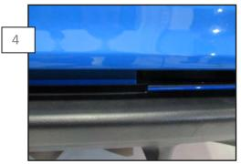
Before removing the tape backing, center the diffuser between the lower reflectors so that you can see how the diffuser sits. Firmly press tape locations from the center of the bumper outward.
