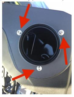
6. Place the Cold Air Box into the engine bay, making sure to line up the bolt opening, the pin (into the rubber grommet), and air inlet into its factory opening. Insert 10mm bolt and tighten.
