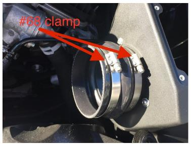
8. Slide the reducing hump hose over the throttle body. Place #48 clamp and #64 clamp
