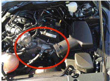
3. Using the 10mm socket wrench, remove the factory air box mounting bolt located in the inner fender. Then life the entire factory air box up and out of the engine bay. Same the 10mm bolt for use later on.
