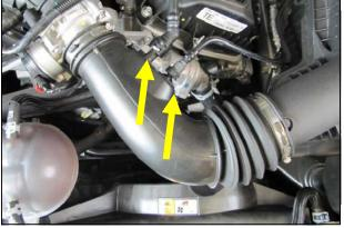
2. Disconnect the 2 breather lines from the intake tube, loosen the hose clamps and remove the factory intake.
