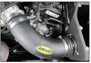
11. Reconnect the breather hoses to the Fittings in the Airaid Intake Tube.
