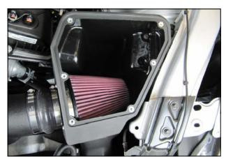
12. Install the Airaid Premium Filter onto the Filter Adapter inside of the Airbox
