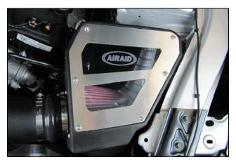
13. Remove the protective film from the Lid and Window before installation. Install the Airbox lid and Window onto the Airbox, with the Window on top, using 6 sets of 1/4" Button Heads. and Washers.
