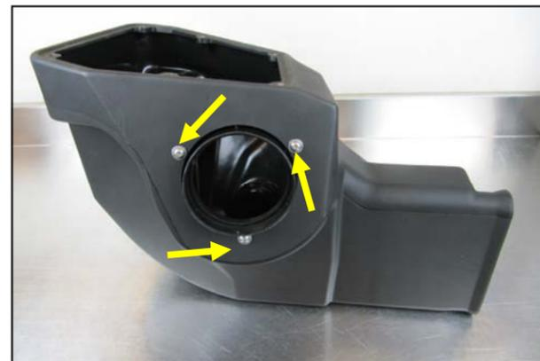
6. Install the Filter Adapter onto the Cold Air Box as shown, using three sets of 1/4-20 Button Head Screws and 1/4" Flat Washers
