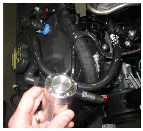
For the Boss intake manifold remove a three inch section of the factory PCV hose and splice in the oil separator as seen below.
