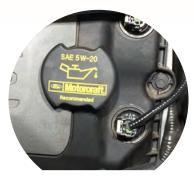
**Oil Cap Installation**: Remove the factory oil cap by turning it counter-clockwise. Then Install the Modern Billet Chrome Oil Cap.
