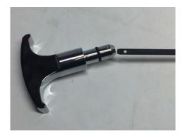
Remove the dipstick from the factory handle and slide it into the Modern Billet Chrome handle.
