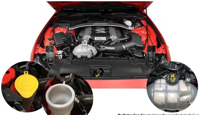
**Windshield Reservoir Cap:** Remove the factory reservoir. Wrap the cable tether around the reservoir opening then press the cap onto the reservoir.
