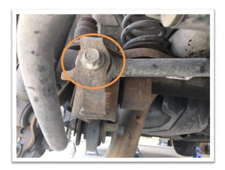
2. On the passenger side, using the same 18mm socket, remove the bolt on the left bracket. Save bolt and nut to reuse. (Note: loosen the panhard support bracket bolt may be necessary to remove the panhard bar.)
