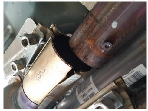
7. Now very gently pick up on the exhaust so the middle hangers pop free from their hole (the bolts you removed in step 3). And then pull the exhaust toward the front of the car so it can slide off of the rear hanger under the bumper. Having a second person makes this step much easier.
