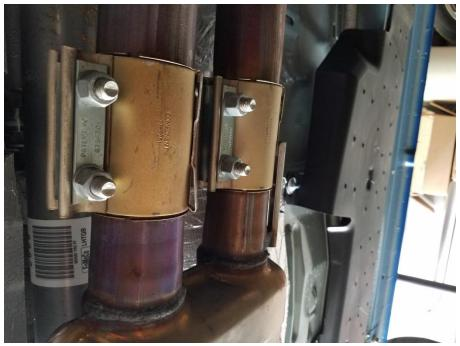
5. Now using the flat head, gently pry the tabs shown so that the clamp can slide over the round nub.
