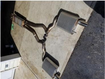
8. Now lay the H pipe on the resonator. You can begin to see where you need to cut the oem piping so it slides all the way into the expanded exhaust pipe section. According to Heartthrob, they want a cut made on both pipes 6" back from the rear of the resonator. I did this and actually found for mine, 6 ½" was needed to allow it to slide back on properly. Cut 6" first and see if that gives you enough.
