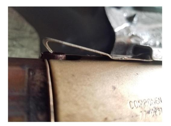
6. Now wiggle and gently pry enough to allow the clamp to slide off of the forward pipe.
