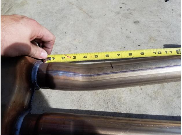
**9.** There is many different tools to cut the exhaust piping. I personally used a cutoff wheel to make a notch and then used a sawzall the rest of the way. Whichever you method make sure to clean up the burrs left behind with a file or deburr tool.
