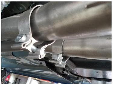
**11.** Go back and tighten all of the clamps as well as the hanger brackets. Start the vehicle and check for any exhaust leaks. Realize you may have a small odor for a few miles. That is just the new exhaust pipes burning off any grease or oils.
