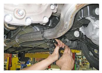
Remove the two (2) 13 mm bolts that retain the exhaust hangers on the IRS sub frame.
