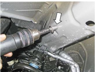
4. Deburr the drilled holes and apply automotive clear coat. Install four (4) rivet nuts (P/N: 95105A191) using the supplied bolt and nut from the rivet nut installation kit (P/N: R1315-5231HWK). Insert the nut onto the bolt and thread the bolt into the rivet nut. Hold the nut with a 17 mm wrench and tighten the bolt nut with a 10 mm socket until the rivet nut is fully seated.
