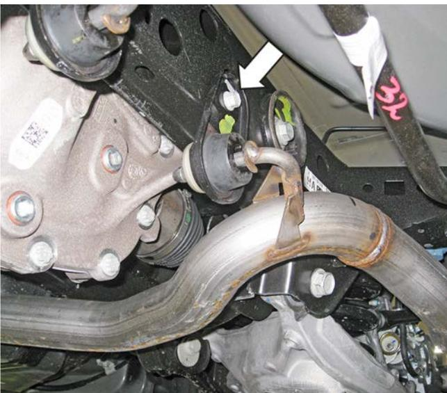
3. Unhook each exhaust hanger from the sub frame and remove each muffler assembly by sliding the inlets down and forward to extract the rear exhaust hangers from their mounts.
