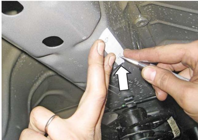
4. Deburr the drilled holes and apply automotive clear coat. Install four (4) rivet nuts (P/N: 95105A191) using the supplied bolt and nut from the rivet nut installation kit (P/N: R1315-5231HWK). Insert the nut onto the bolt and thread the bolt into the rivet nut. Hold the nut with a 17 mm wrench and tighten the bolt nut with a 10 mm socket until the rivet nut is fully seated.
