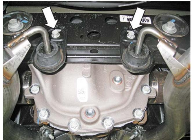
8. Install each side of the ROUSH exhaust system by inserting the rear exhaust hangers first and then sliding each side forward to fully seat the inlets with the forward section of the stock exhaust. Be sure to connect the rubber isolators to the hangers that were installed in step 7 and also reinstall the two (2) IRS sub frame exhaust hangers with the two (2) 13 mm bolts that were removed in step 2 and torque to 18 lb-ft (25 Nm). Torque the exhaust pipe clamps to 35 lb-ft (47 Nm).
