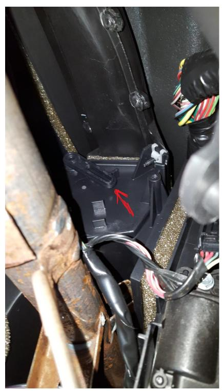
**Step 4:** Make very sure to realign the arm of the new motor and the holder carefully and then insert the old 8mm screws from the old motor back in the same two locations.
