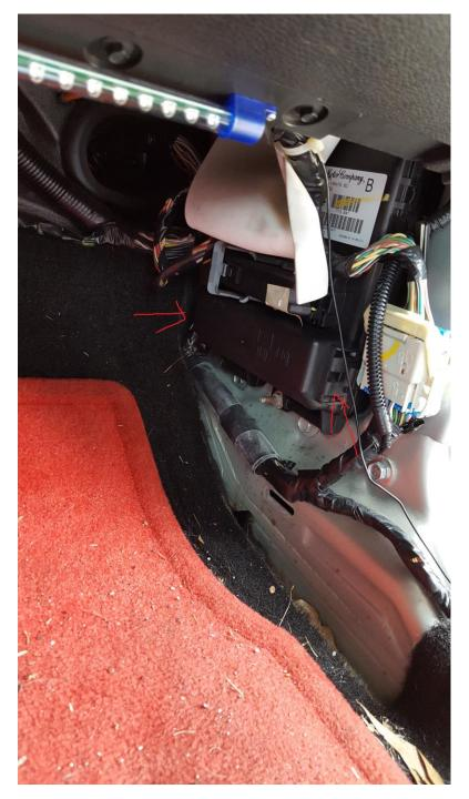
**Step 5:** Remove the plastic trim around the inner fuse box.
