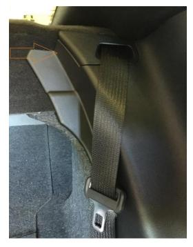
5. With these out, remove the two interior side panels from the car. You can pull these away, tab by tab, starting from the rear, exerting enough force to pop out each one as you move along back to front.
