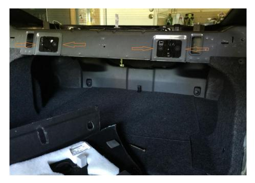
10. After the hooks have been removed, and with the carpeted area out of the car, use your box cutter blade or scissors to trim away a small portion of the area covering the hole you will need to access. **NOTE**: there are holes on each side of the black hook you have removed. Ensure that you are cutting a spot to reveal the hole facing the **exterior** of the car, rather than the interior. See picture below:
