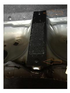
13. Locate the driver's and passenger's side support brackets from the kit. Align them over the stock bolt holes and pins in the pictured location – use the labeled bolts from the kit to secure the brackets:
