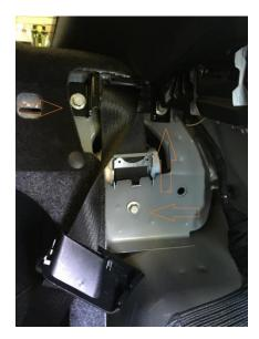
7. With these out of the car, you will need to remove the seatbelt from the plastic trim piece that you will be reinstalling into your car. Use a box cutter or similar tool to make a small slit at the upper rear so that you can slide out the seatbelt. **AIM THE BOX CUTTER TOOL AWAY FROM YOUR BODY!** Once removed, set these plastic pieces aside to reinstall after you replace the side panels in a later step.
