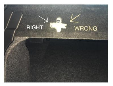
11. With this piece trimmed, you can reinstall the upper carpeted area into the car. Once that has been replaced, reinstall the factory side panels into the car, and push the modified seatbelt holders back into place in their original locations, as well.
