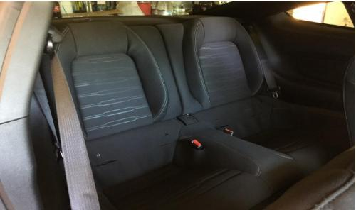
1. You will need to remove the stock rear seats. Begin by feeling around under the middle of each rear seat and locating the release button. Depress the button and lift up on the lower section of the seats. There is one button on each side. Note the hole locations in the bottom centers below:
