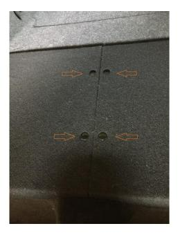
15. Now, place the upper rear portion of the kit into the car, and align it into place. Use the two included push pins to secure the panel into the holes you revealed in step # 10.
