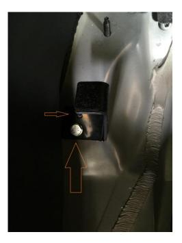
14. You can now install each section of the lower rear seat delete. Use four of the six included push pins to secure the two sections to the new center brace piece. Two pins are extra, in case of breakage.
