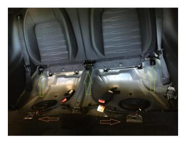
2. Locate the bolts along the bottom sides and middle that are holding the upper rear seat section in place. Use a 3/8in Socket wrench with 15mm socket to remove the three bolts, noted by green arrows
