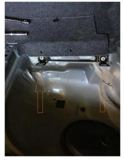
9. Now, carefully lift up and remove the carpeted upper rear deck panel. With this removed, use a T40 torx bit to unlatch the two black hook pieces that hold the stock upper rear seat.
