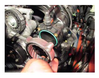
Step 5: Torque the supplied bolts to 10-12ftlbs. And reinstall the remaining parts in
