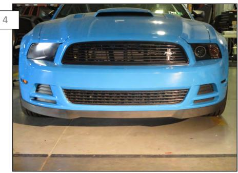
Attach the MMD chin spoiler with the factory hardware. Center the lip. Then apply firm pressure to tape surfaces. \*\*Note: the factory splash shield mounts under the chin spoiler. If it is mounted between the chin and the bumper you will create a gap.
