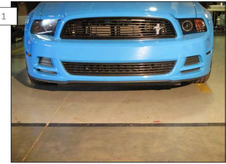
Start by removing the factory lip. \*\*Note: supporting the front of the car with jack stands is not necessary but it can be helpful.
