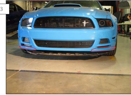
Prep the bumper with alcohol wipes where the tape on the lip will contact the paint. Use the adhesion promoter on the exposed tape surface.
