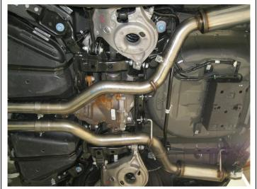
**Step 3.** Next attach the Extension Pipe Assemblies to the X-Pipe using the supplied 3.00" clamps and fitting the hangers into the rubber insualtors.
