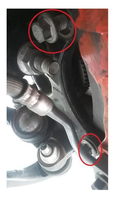
**4.** Take one of your zip ties and run it through one of the holes in the body just above the front sub frame (circled in red in picture below), you will use this to hang your caliper from. Once you have done this you can now remove the top caliper bolt and slide the caliper off the rotor. Put the zip tie through the top bolt hole on the brake caliper and secure it. This will prevent damage to your brake hose from supporting the weight of the caliper.
