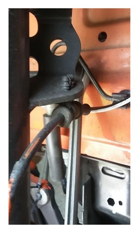
7. Remove the sway bar end link where it attaches to the front strut. You will need an 18mm deep socket to remove the nut (circled in red). There is a hex on the back of the end link bolt that you will need to hold with your 17mm wrench while you remove the nut (pictured below). Once the nut is removed, remove the end link from the strut and move it out of the way.
