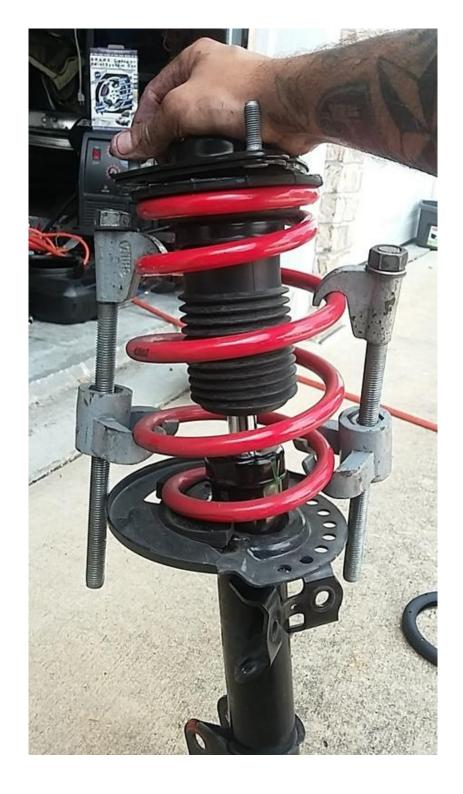
12. Tighten your compressor until there is no pressure from the spring against the strut mount. Next loosen (but do not remove) the strut shaft nut (circled in red below) with a 21mm socket. The spring should not decompress as you loosen this nut, if it does you haven't fully compressed the spring and need to do so before going any further. This is where people can get seriously injured if they don't do things right.
