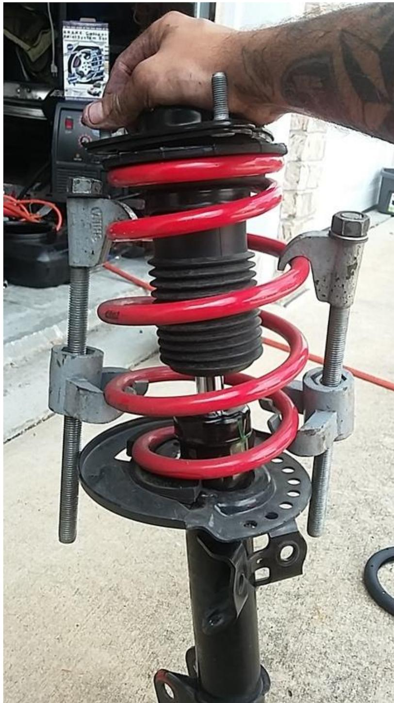
12. Tighten your compressor until there is no pressure from the spring against the strut mount. Next loosen (but do not remove) the strut shaft nut (circled in red below) with a 21mm socket. The spring should not decompress as you loosen this nut, if it does you haven't fully compressed the spring and need to do so before going any further. This is where people can get seriously injured if they don't do things right.
