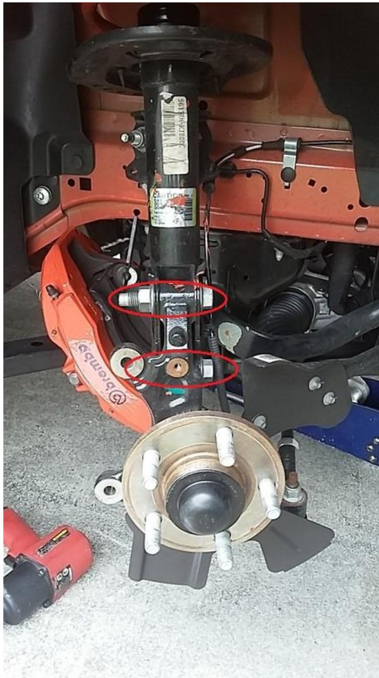
9. With the nuts on the end of the bolts, hammer them out with your hammer. Ensure that the nuts are far enough on the bolt shaft, otherwise hitting them could damage the threads. You can remove the bolt by hand once the splines are visible (pictured below).
