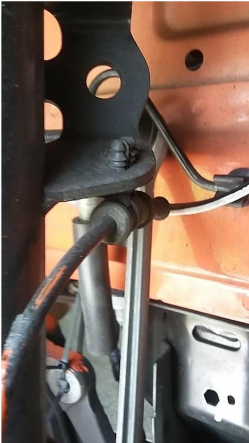
7. Remove the sway bar end link where it attaches to the front strut. You will need an 18mm deep socket to remove the nut (circled in red). There is a hex on the back of the end link bolt that you will need to hold with your 17mm wrench while you remove the nut (pictured below). Once the nut is removed, remove the end link from the strut and move it out of the way.
