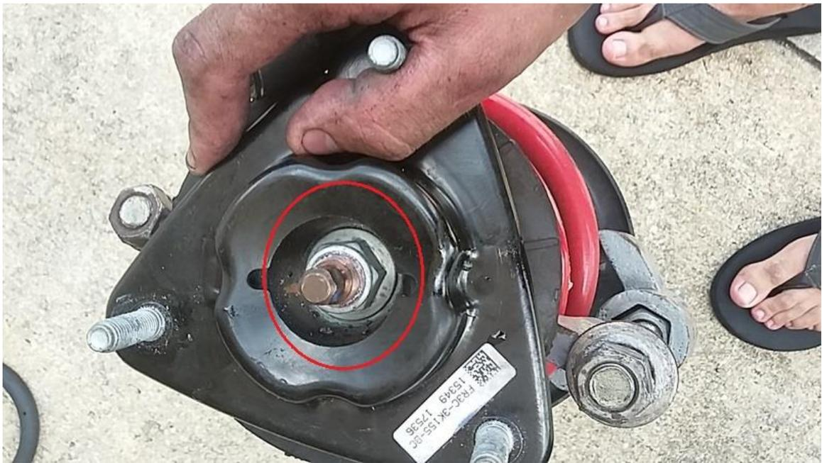
13. Once you are sure the spring is fully compressed, you can remove the strut shaft nut the rest of the way and then remove the strut mount from the strut assembly.
