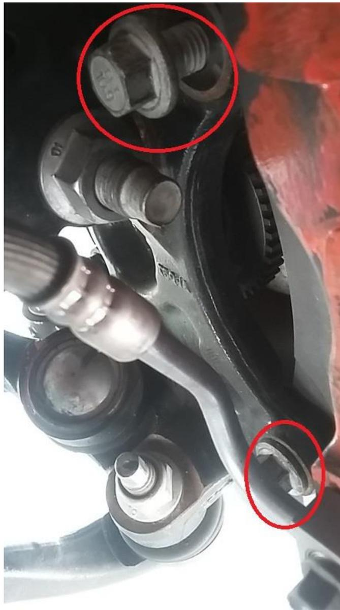
4. Take one of your zip ties and run it through one of the holes in the body just above the front sub frame (circled in red in picture below), you will use this to hang your caliper from. Once you have done this you can now remove the top caliper bolt and slide the caliper off the rotor. Put the zip tie through the top bolt hole on the brake caliper and secure it. This will prevent damage to your brake hose from supporting the weight of the caliper.
