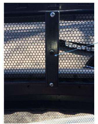
Step 10:. Using the 6 silver screws attach the grille to the bumper as shown in the example photos.
