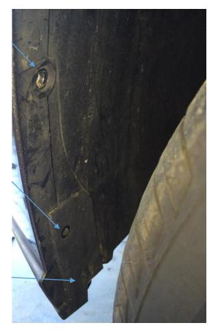
Step 4: Remove the 11 screws along the bottom of the grille. After this step the bumper is no longer attached with screws, it is held on only by clips.
