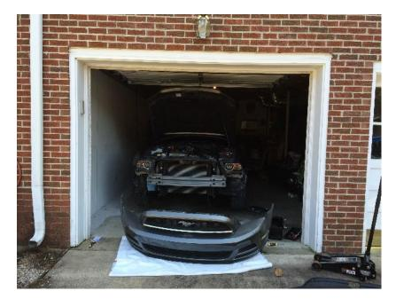
Step 7: Remove the stock grille from the bumper. To do so, push on the grille from the back of the bumper while simultaneously applying pressure to the locking pins.
