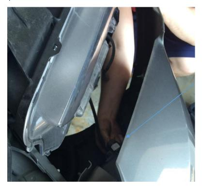
Step 6: Pull the bumper off of the car by removing the bumper at the wheel wells first, then by pulling the bumper away from the car.
