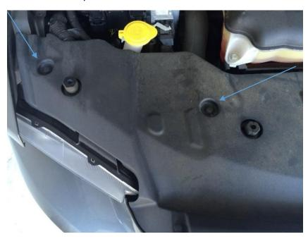
Step 2: Remove the 4 plastic push pins and 4 silver bolts from the top of the bumper.
