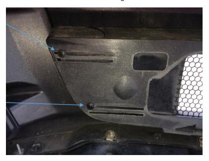
Step 10: Attach the screen to the grille. Use the pictures below as reference. You are going to place 2 screws on the top and two screws on the bottom in order to attach the screen.
