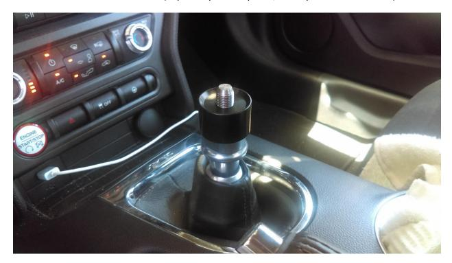
**Step 3:** Thread on your new shift knob until it reaches your desired position and then rotate the lock out collar COUNTER CLOCKWISE until it meets the bottom of the shift knob
