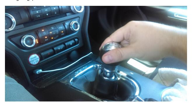
Step 2: Thread on reverse lock out collar (Separate piece required; sold by AM item# 389115)
