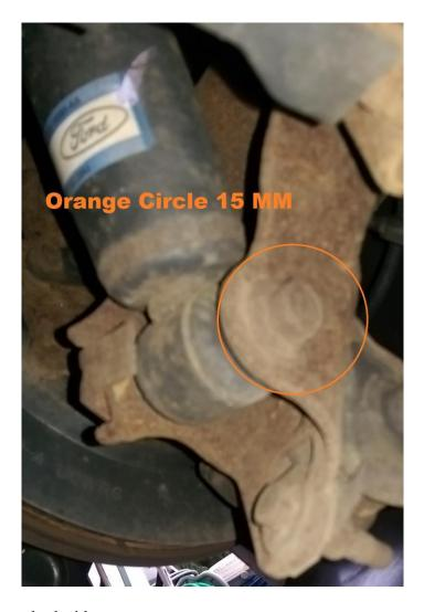
Step 8 Remove shocks on both sides.
