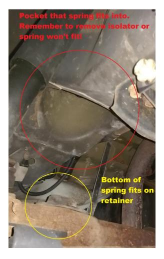
Step 13 Raise axle with jack so that there is a slight amount of compression on the spring holding it in place.
