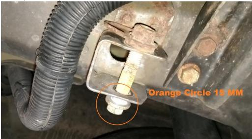
Step 7 Use 15 mm socket to remove shock bolts. Shocks will expand after bolt is removed. (See Below)
