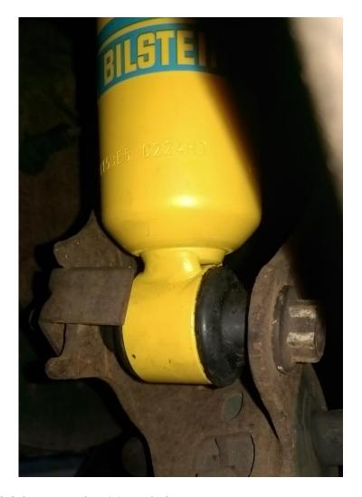
Step 17 Reinstall and tighten sway bar 15 mm bolts.
