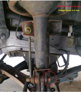
Step 5 Remove brake line from strut using 10mm socket. (See Below)
