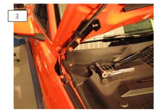
Slide the bracket between the loosened hood nut, and the hood hinge. Then reinstall remaining hood nut. \*\*Note: Passenger side bracket will require you to remove the windshield washer hose retaining clip.
