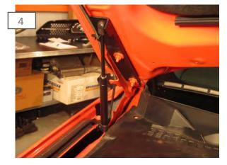
Install supplied gas strut onto mounting brackets.
