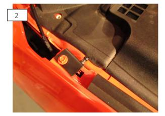
Re-install fender bolt through the lower strut mount bracket.
