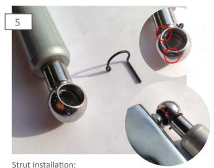
Remove the retaining clip. Place strut on the ball stud. Then reinstall the retaining clip. \*\*Note: Make sure the retaining clip slides all the way through.
