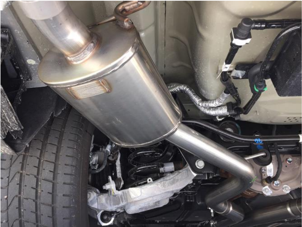
Figure 2d Completed ARH system installed showing ARH muffler and tail pipe.
