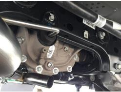
**Step 7:** Once the muffler is hanging, bolt in the hangers with the 13-millimeter sockets and ratchets until snug, and then tighten the clamp connecting the muffler pipe and the H pipe with a 15-millimeter socket until tight. Take this time to align everything up until the consumer is happy, and then tighten down all 13 millimeter hangar bolts and exhaust clamps (DON'T FORGET THE H PIPE IN THE STOCK CLAMPS)-Repeat for the opposite side.
