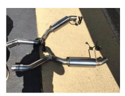
**Step 6:** Insert the H pipe into the stock clamps where the resonator was using something to prop up the other end and using a 15 millimeter socket and ratchet tighten the clamps down until its snug.
