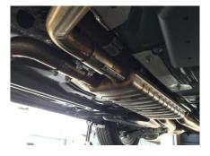
**Step 3:** Take a 13 millimeter socket with a ratchet and remove the bolts holding the exhaust hangars in place, starting with the hangars near the rear differential (use the extension to remove the lower bolt on the muffler hangars)
