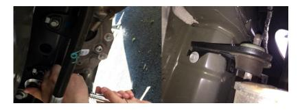
**Step 4:** After the bolts are removed prepare to remove the exhaust from the mufflers by pulling the system toward the back of the car, before doing so, there is 1 hook on each hangar that needs to be lifted out of where it is resting in. Once the hooks are removed tug the exhaust toward the back of the car and the resonator will slide free and the exhaust will come loose, **BE CAUTIOUS WHEN PULLING BECAUSE THE RESONATOR WILLFALL ONTO THE GROUND UNLESS YOU HAVE HELP.**
