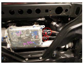
Step 3: Loosen the lock nut. Remove tie rod nut. Using a Tie Rod removal tool separate the outer tie rod from the wheel knuckle.
