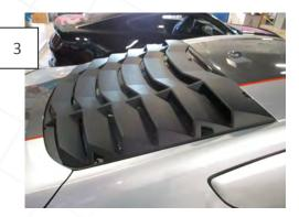
Peel the backing from the adhesive tape on the brackets and apply some of the 3M Adhesion Promoter to the tape. Using a partner, place the louvers over the rear window aligning the tope edge of the louver with the top edge of the glass..
