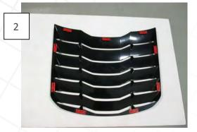
Lay the louvers upside down on a surface that will not scratch the finish. Install the 8 brackets as shown and install the nuts finger tight. You just want to tighten the brackets enough so they stay in place; there is no need to fully tighten them at
