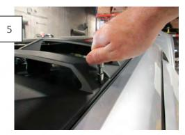
Once the sealant has cured, install the louver onto the brackets using the supplied washers and closed end nuts. Use an 8mm socket and ¼ drive ratchet to install the nuts just past finger tight. Do not over tighten the nuts as you will risk damaging the studs.
