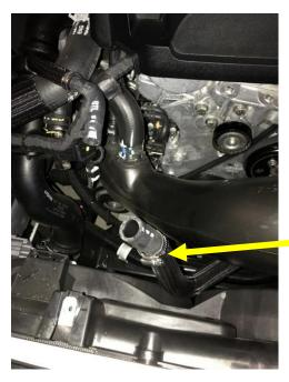
Place the worm drive clamps on the hoses, ensuring they are positioned to finish where you want
