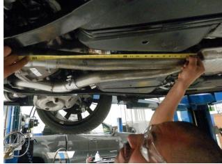
**Step 1.** Begin removing the OEM exhaust system by cutting both pipes exiting the resonator. Measure and cut 23.5" (driver side) and 24.5" (passenger side) from the rear of the resonator. Next, extract the hangers from the rubber insulators and remove the OEM mufflers. Retain insulators as they will be used to install the new system.
