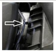
Unplug the air temp sensor from the air box. Detach the air temp Sensor wire harness from the side of the air box by slightly pulling on the harness on the barbed mounting pin.
