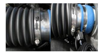
Install the rubber o –ring into the adapter pipe, remove the Air Temp sensor from the stock air box and install it into the adapter tube. Install the BBK adapter tube into the inlet tube. Install the BBK coupler and supplied clamps onto the BBK air filter, install the BBK Air Filter thru the hole in the air shield. Next slide the air filter onto the adapter tube once you have it in position tighten down all of the clamps.
