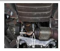
Loosen the 2 bolts that connect the down pipe to the cat back portion of the exhaust. Remove the rubber exhaust mount from the chassis. This mount will be reused to install the BBK High Flow downpipe.
