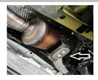
Unbolt the downpipe support bracket from the down pipe.
