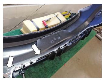
33. Apply 3M Ad-Pro® (P/N: 021200-27571) onto the rear edges of the side valance pieces (P/N: 1315-17F955 & 1315-17F956) and then install the 2-sided tape (P/N: TAPE-015-12.5x68).
