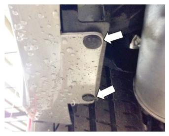
Remove two (2) 7 mm screws and two (2) push-in retainers on the LH and RH sides under the rear bumper.
