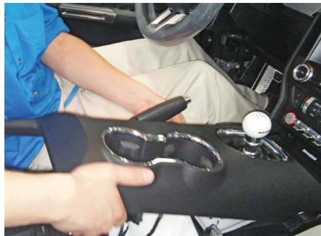
27. With the emergency brake fully engaged, lift the top portion of the center console up and unplug the connectors for the key fob detection circuit and for the cup holder lighting (if equipped).
