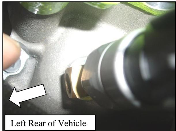
13.a. Install the boost gauge fitting into the port facing the left rear of the vehicle. Tighten the fitting to 10 Nm. Position the fitting so it is pointing downward and toward the left rear of the vehicle. Install the boost gauge line removed in step 10.a onto the boost gauge fitting. Route the boost gauge line so it is clear of moving and/or hot engine components.
