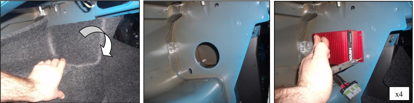
4. With a 1/8" drill bit, drill four (4) pilot holes in the locations marked in step 3. Using a 1/4" socket, install the FPVR using the four (4) supplied screws (R07030003-13-AA).
