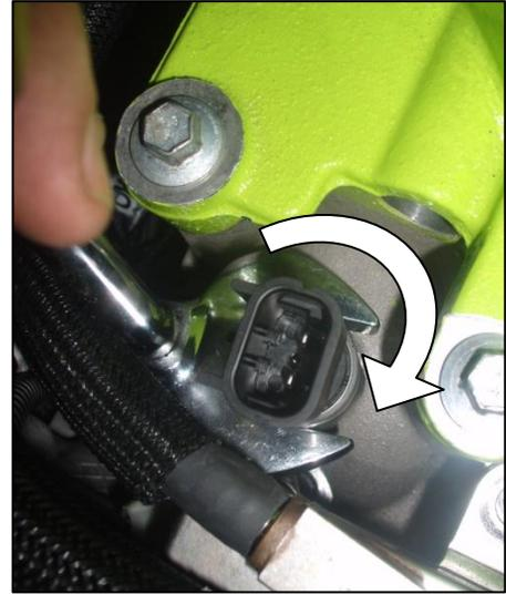
12.b. Following factory wiring, route the harness along the back of the engine to the passenger rear side of the intake manifold. Plug the connector into the switch installed in the previous step.
