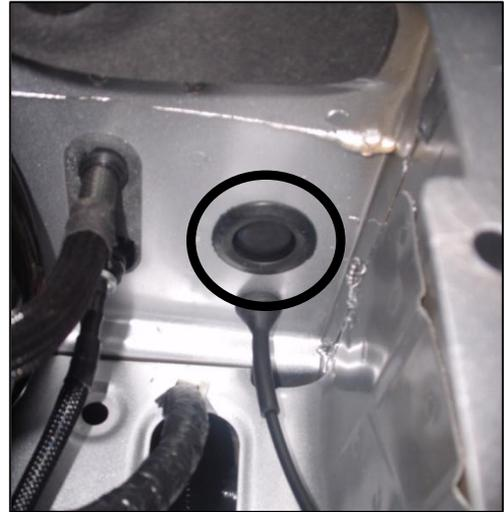
10.b. Pass the intermediate harness through the firewall and into the engine bay. Seat the grommet into the open port on the fire-wall.
