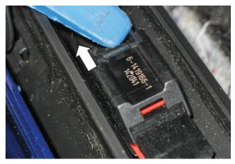
After feeding the removed clip between the weatherstrip and the vehicle body, remove the OEM sill panel. This completes the removal process.
