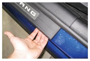
Once the clips have been lifted, use a plastic pry tool/fiber stick between the silver "Mustang" panel and the body of the vehicle to remove the taped panel without damage.
