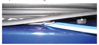
Remove the trim panel next to the seat. This can be done independent from the weatherstripping. Fit your fingers around the bottom-front edge of the trim panel and pull upwards. The panel is retained by four (4) clips as shown below.
