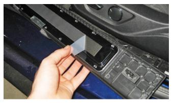
**NOTE:** Once the sill panel is clipped into place, remove the blue protective covering on the illuminated "ROUSH" logo.
