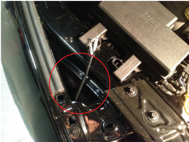
Step 8 Fish the vent harness up behind the headlight into the fender.
