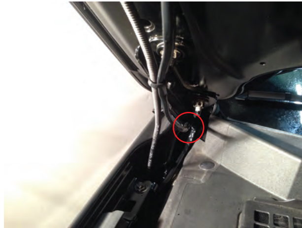
Step 10 Zip tie the wiring harness to base of the hood hinge. Make sure the harness is out of the way of hinge when it closes.
