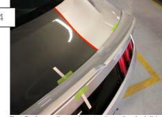
Test fit the spoiler and center it on the deck lid. Then tape the template to the deck lid where they lay. Carefully remove the spoiler from the templates. \*\*Note: this is the most important step so that the holes are drilled in the correct place.
