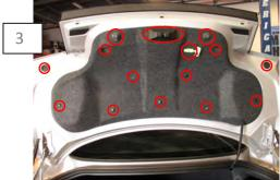
Remove the deck lid panel. There are various push pins, the rubber bumpers located at the top unscrew. I was able to sneak the liner off by manipulating it around the latch trim.
