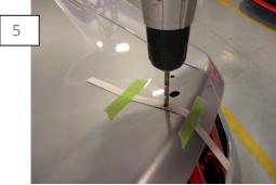
Once the spoiler is removed, carefully drill the center of the template holes. Finish with a 7/32's drill bit. \*\*Note: Use nail polish to cover any exposed metal to prevent rusting.
