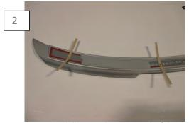
Center all 4 drilling templates over each of the 4 mounting points.
