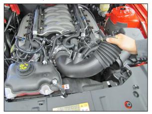
8. Loosen the hose clamps securing the factory intake tube and remove the intake tube from the
