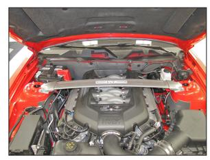
17. Reinstall the strut tower brace and secure with the factory nuts.
