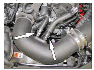
15. Connect the crank case vent hose and EVAP vent hose if equipped to the quick connect fittings as
