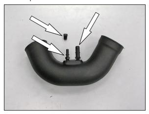
13. Install the provided quick connect fittings into the K&N intake tube as shown.
