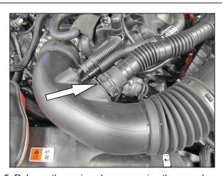
5. Release the spring clamp securing the sound tube to the intake tube and then disconnect the sound tube from the intake tube. Remove the sound tube from the vehicle.
