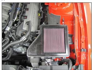
TO. Remove the factory all litter and replace with the provided K&N® air filter, then reinstall the air
