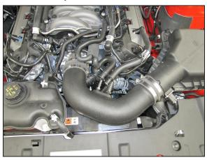
14. Install the K&N® intake tube into the hose at the air box and then into the hose at the throttle body. Adjust the tube for proper fitment and then secure with the provided hose clamps.
