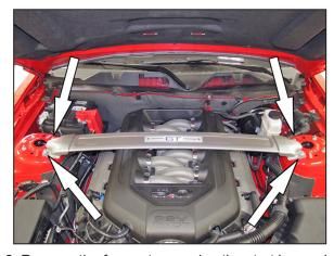
2. Remove the four nuts securing the strut bar and then remove the strut bar from the vehicle.
