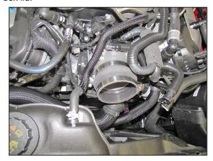
11. Install the provided coupling hose (08699) onto the throttle body and secure with the provided hose
