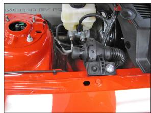
6. Install the provided cap onto the sound drum as shown.
