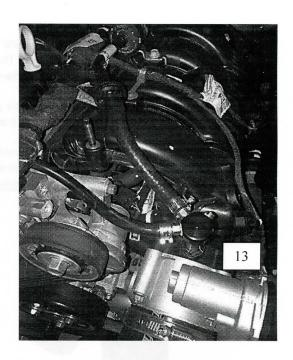
14. Locate the factory BOV and unplug the solenoid plug.
