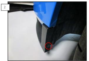
Begin with removing the bottom most factory bolt on the bumper trim. Screws will be reused.
