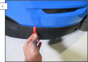
Remove the tape backing off the center of the chin spoiler. Peel the outer edges slightly as seen above. Once the Chin is fitted. Remove remaining tape backing and apply firm even pressure on all taped surfaces. Reinstall the factory screws.
