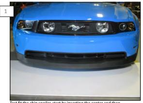
Test fit the chin spoiler, start by inserting the center and then manipulate the either end to tuck around the back of the bumper.
