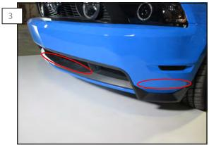
Prep any and all contact points using the supplied alcohol wipe. This is critical for a secure fit. Once clean, apply the provided adhesive promoter to the tape surfaces.
